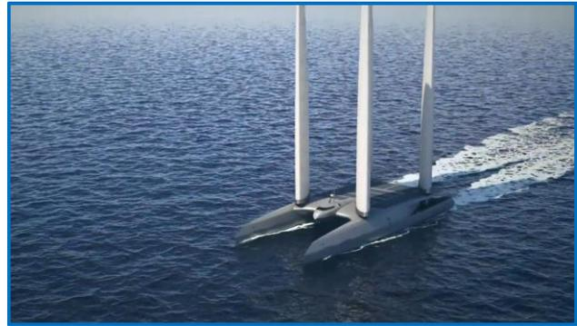
The Drift project. Rated power 1-2 MW, Length 58 meters, H<sub>2</sub> Production 150 t/a. Credit to <https://drift.energy/> (UK).
